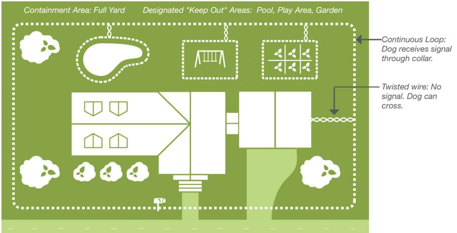
The SmartFence™ Transmitter sends a coded **digital FM radio signal** through a wire buried in your yard (the boundary wire). The wire is buried 3-4" beneath the surface of the yard or can lie on top of the ground (e.g. in wooded or rocky areas.) **It is not electrified**, so it can also be installed in water (streams, in lakes, etc.)
