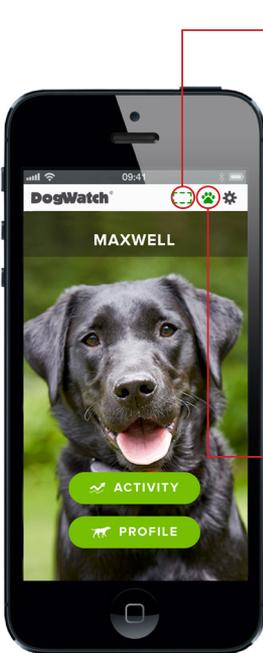
The Loop Icon indicates **Transmitter and Boundary Loop** status
